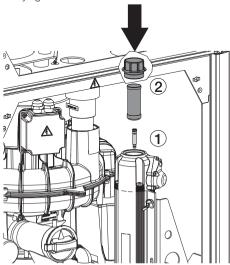
Connect the drying unit to the compressed air hose coming out of the cooler.
