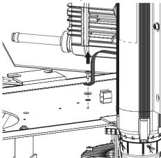
> Remove the clip for L bracket.
