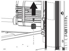
Mount the valve block with earth strap.
