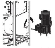
Mount the compressor unit on the retaining plate using four nuts.
